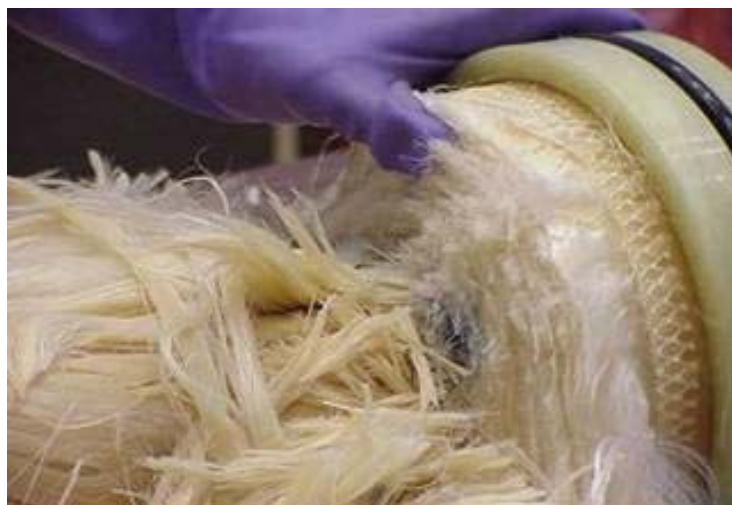
Fig.2 Photograph of the feed side of a HFF membrane. The interior black spot is due to Sulfate Reducing Bacteria and the brownish color is due to fouling
