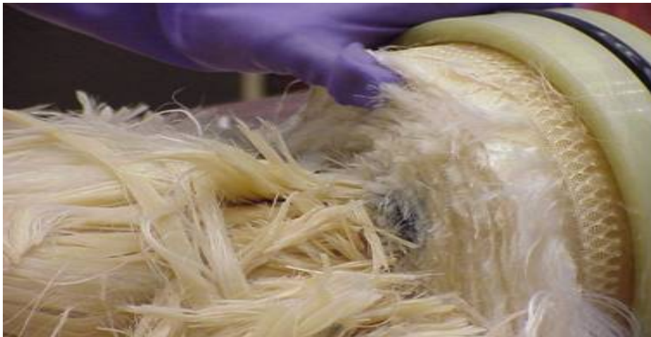
Figure 4. View of autopsied CTA membrane showing a black colored stain near the feed tube
