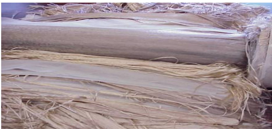
Figure 5. View of autopsied PA membrane showing the color difference among the fibers
