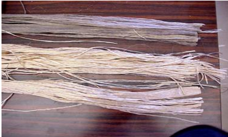
Figure 6. View of PA membrane fibers showing the color difference among the fibers
