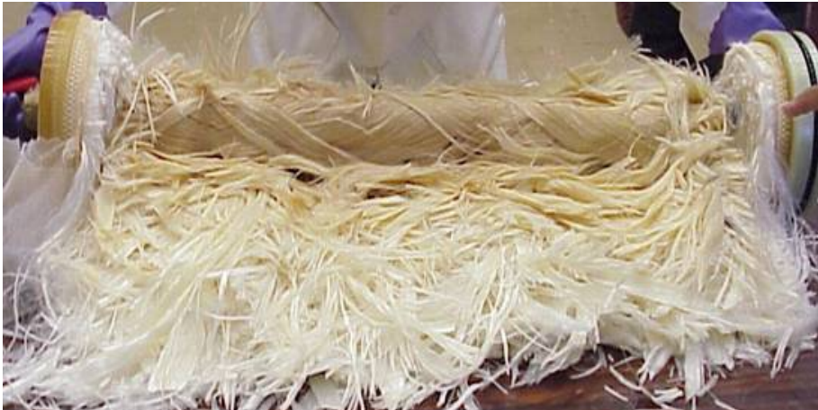
Figure 3. View of autopsied CTA membrane showing the color difference among the fibers
