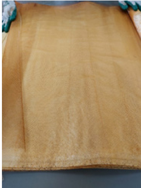
Figure 45 Membrane Autopsy conventional operation
