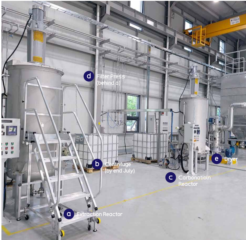
Demonstration Pilot for Vaterite-type CaCO 3 production under assembly in South Korea
